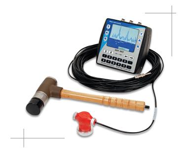
The Slab Impulse Response (SIR) system is designed to identify subgrade voids below slabs-on-grade less than two feet thick. In addition, the Slab IR test method can be used on other concrete structures to quickly locate areas with delaminations or voids in the concrete, if the damage is relatively shallow. Slab IR can be performed on reinforced and non-reinforced concrete slabs as well as asphalt or asphalt-overlay slabs.
