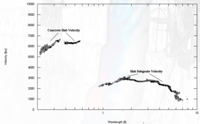
The figure below shows dispersion curves determined from SASW measurements on asphalt pavement. The shift of the surface wave velocity (or modulus) curves is due to changes in temperature. The SASW measurements also determined the thickness of the surface layer.
