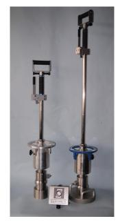
Larry Olson introduced this innovative concept to the University of Maryland as a result of experiments with the Olson Instruments Light Weight Deflectometer in an effort to find an easier, cleaner, less expensive alternative to the Nuclear Density Gauge. As a result of this study, Olson Instruments has developed the LWD-LAB unit to be used for this purpose.
