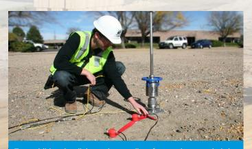
Two additional radial geophones allow for two layer analysis by AASHTO Odemark Method of Equivalent Thicknesses approach
