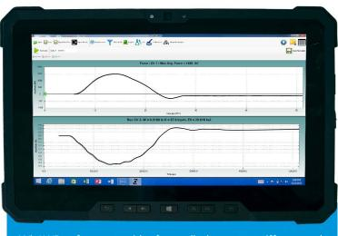
WinLWD software provides force, displacement, stiffness, and modulus values in real time during field and laboratory testing.
