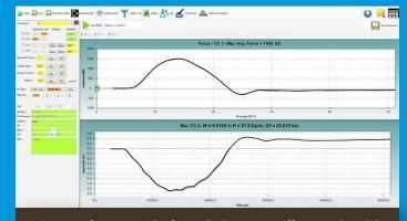
WinLWD software provides force, displacement, stiffness, and modulus values in real time during field and laboratory testing.
