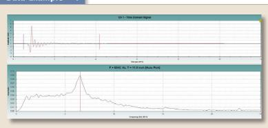
Performing the IE method at a sound concrete location gives results similar to the figure shown. A single, clear peak representing a known thickness is indicative of sound concrete. The slab investigated was 11 inches thick and the bottom echo results in a peak at 11 inches.
