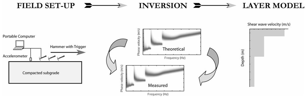
**Figure 2. MISW process schematic showing data acquisition, processing and shear wave velocity profile output.**
