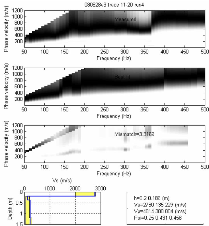
**Figure 7. MISW Matching of Phase Velocity Spectrum for Experimental (top) and Theoretical Best-fit (2<sup>nd</sup> plot), and Mismatch (3<sup>rd</sup> plot) with MISW Theoretical Shear Wave Velocity Profile vs. Depth (left-bottom) and Layer Information (right-bottom).**
