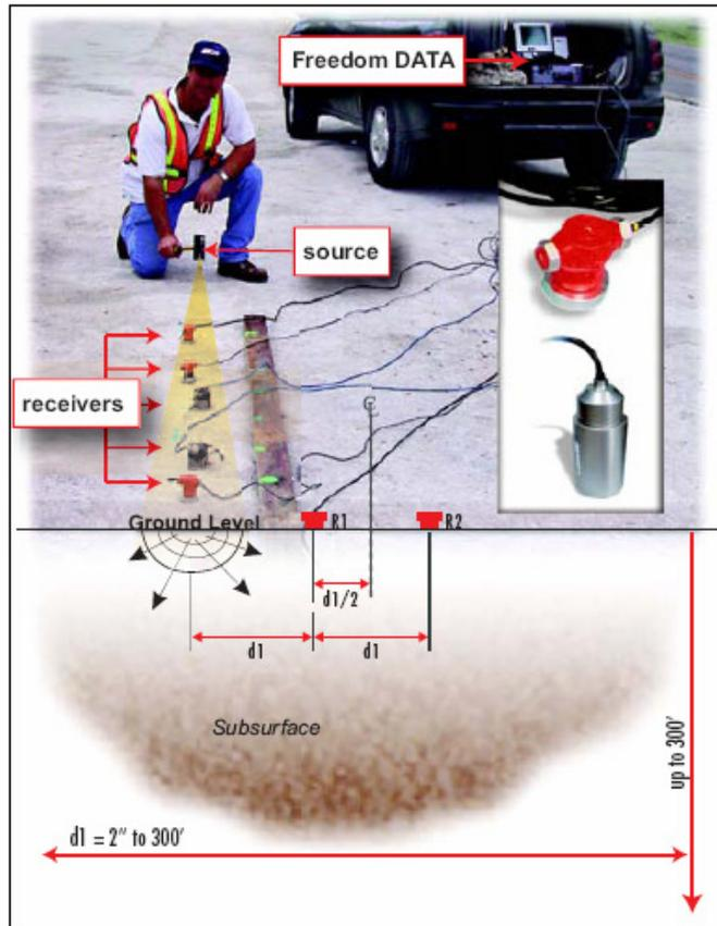
Figure 1. SASW testing with geophone receivers and an impact hammer source.
