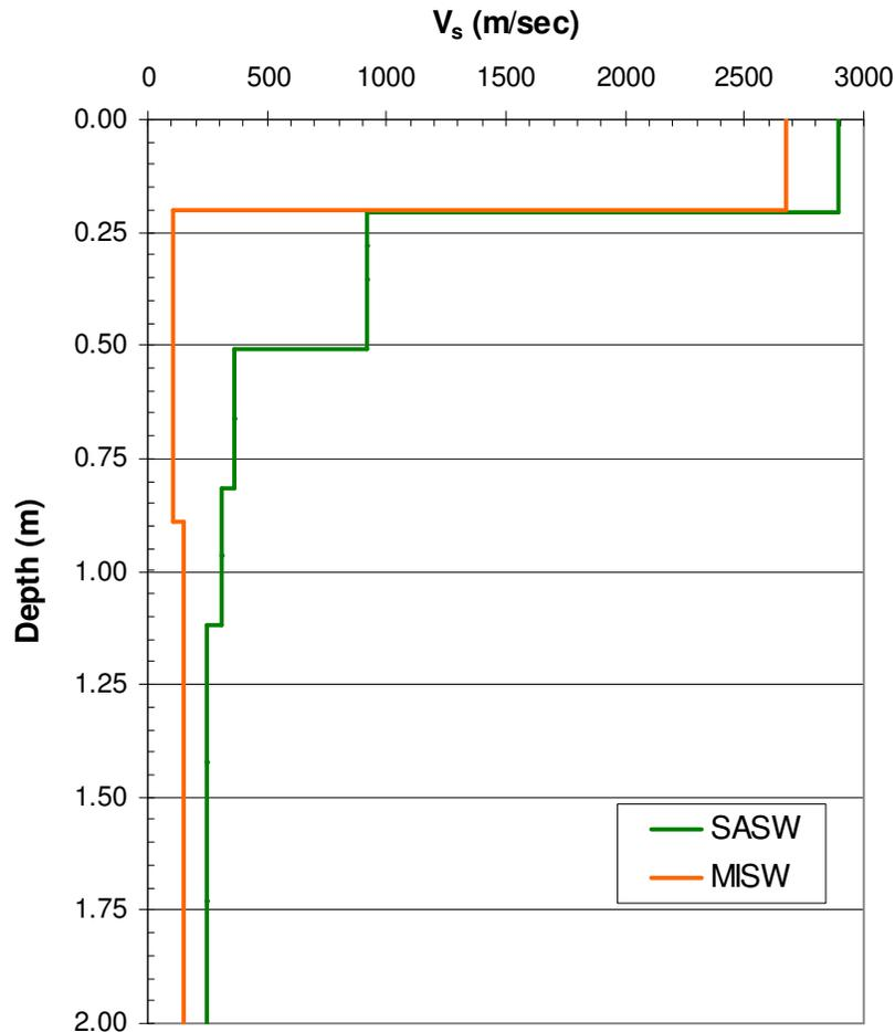
**Figure 8. Comparison of SASW and MISW shear wave velocity profiles with depth. Example data from 1 of 9 similar sites.**
