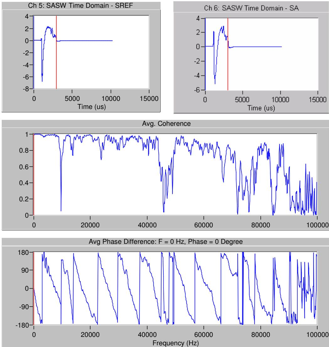
**Figure 3. Example SASW data plot: time domain data of geophone (top plot), coherence for data quality (middle plot), and phase transfer function between geophones (bottom plot).**
