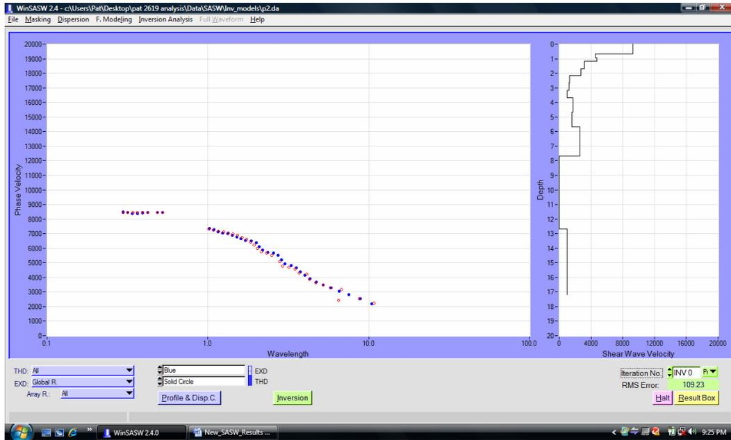
**Figure 5. SASW dispersion curve plot for Concrete Pavement Site (phase velocity vs. wavelength on left with good match of experimental data – open circles and theoretical match – solid circles) and Theoretical Shear Wave Velocity vs. Depth on the right.**
