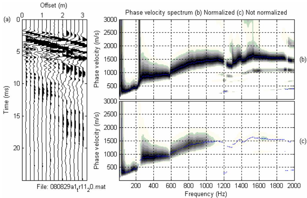
**Figure 6. Example MISW results from Concrete Pavement Site with time domain data in left plot and Phase Velocity Spectrum in right plots.**
