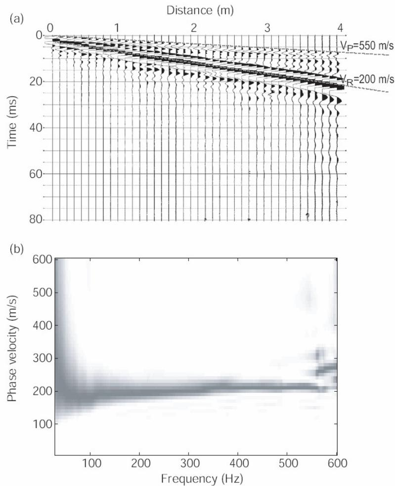
**Figure 4. Example MISW data plot: time domain data of receiver (top plot) from left to right each trace from increasing impact to receiver distance, and the dispersion curve image showing phase versus frequency (bottom plot) – note this example data is from a separate project on natural soils to illustrate simple, single layer data.**
