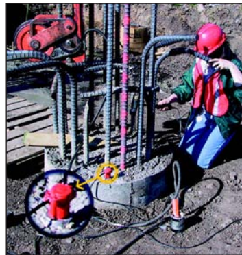
Performing SE/IR evaluation on a drilled shaft top
