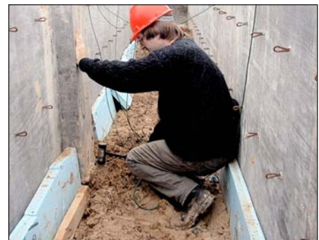
Performing SE/IR evaluation on concrete foundation walls
