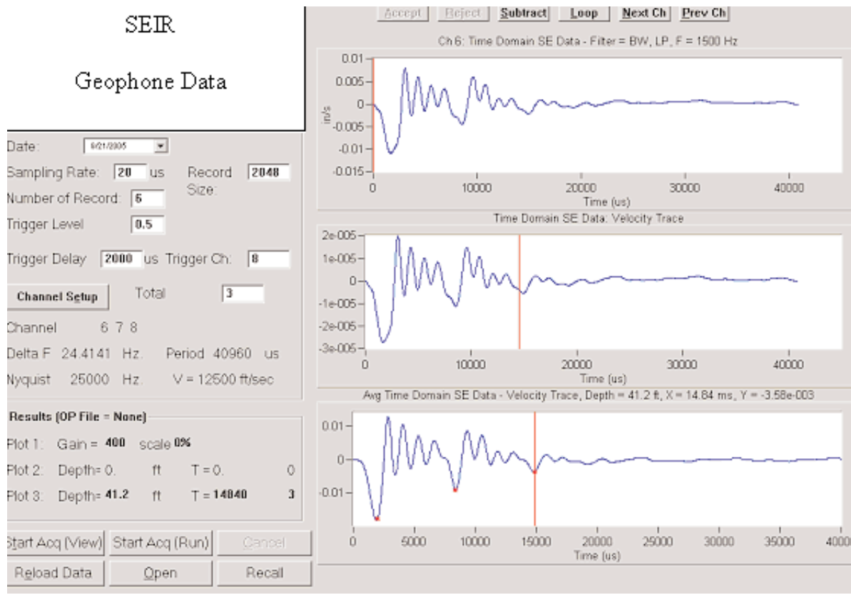
Figure 3. SE/IR results showing good quality Sonic Echo (SE) geophone data
