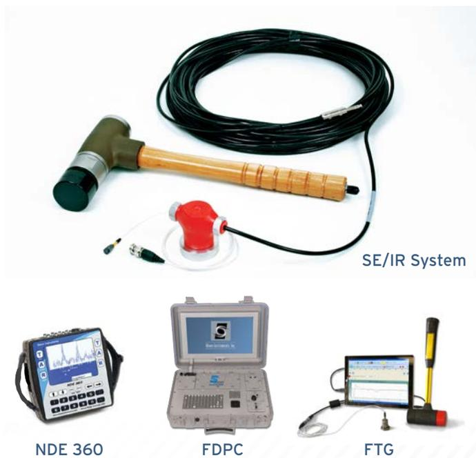
functions, in order to optimize reflections coming from the bottom of the foundation and to reduce the effect of high-frequency surface waves. In IR tests, the time records of the hammer and the receiver are transformed to the frequency domain. The transfer and coherence functions are then automatically calculated by a digital analyzer.
