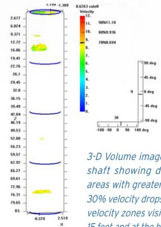
*3-D Volume image of a shaft showing defect areas with greater than 30% velocity drops. Low velocity zones visible at 15 feet and at the bottom*
