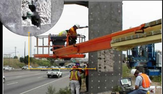
**2-D VELOCITY TOMOGRAM OF COLUMN** identifies slow velocity zones indicative of internal poor quality concrete due to poor consolidation in a horizontal slice and good concrete
