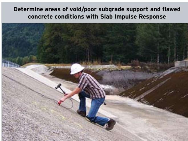
Determine areas of void/poor subgrade support and flawed concrete conditions with Slab Impulse Response
