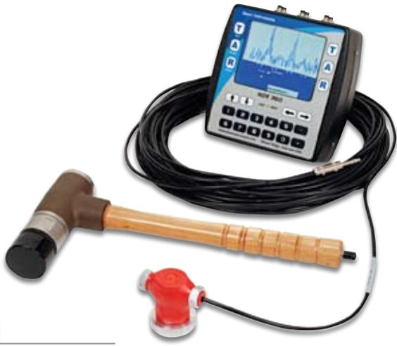
**The Slab Impulse Response (SIR)** system is designed to identify subgrade voids below slabs-on-grade less than two feet thick. In addition, the Slab IR test method can be used on other concrete structures to quickly locate areas with delaminations or voids in the concrete, if the damage is relatively shallow. Slab IR can be performed on reinforced and non-reinforced concrete slabs as well as asphalt or asphalt-overlay slabs.
