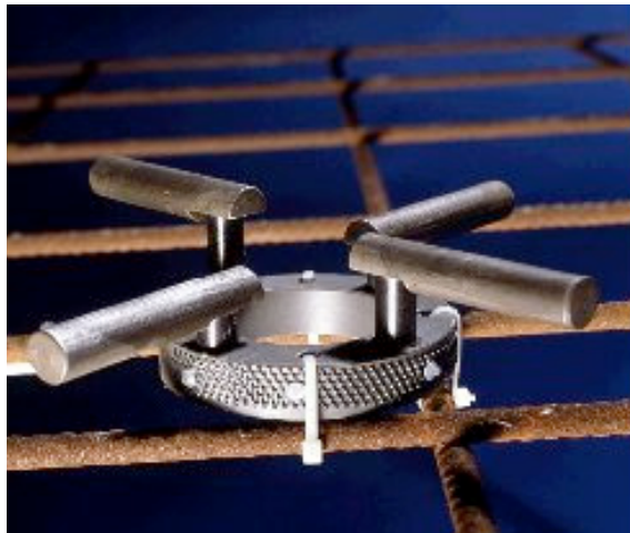
The CorroWatch attached to the reinforcement
